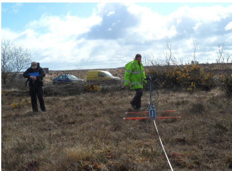
Figure 5.3: GSSI Multi Low Frequency antenna in operation at 80MHz.
