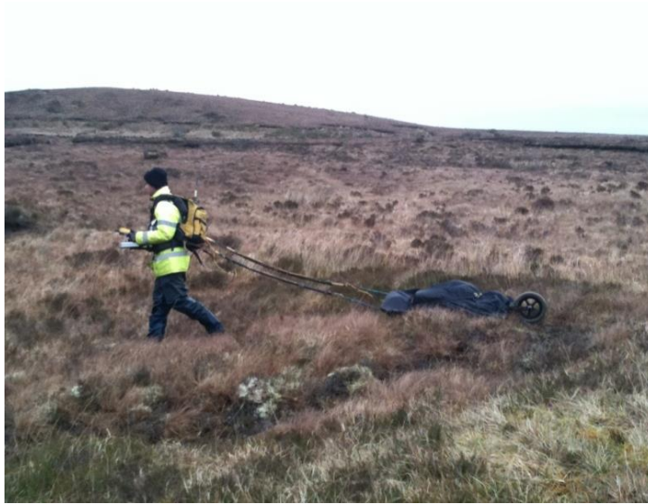
Figure 5.2: GSSI SIR 3000 system being operated with hand dragged 250MHz antenna.
