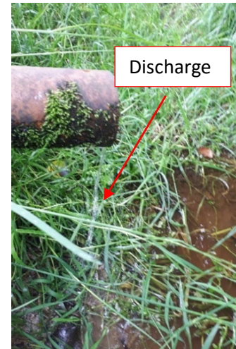
Figure June 5.4-3 (Right). PD GW flow 24 th June 2020. Flow Rate = 0.02 litres/sec.
