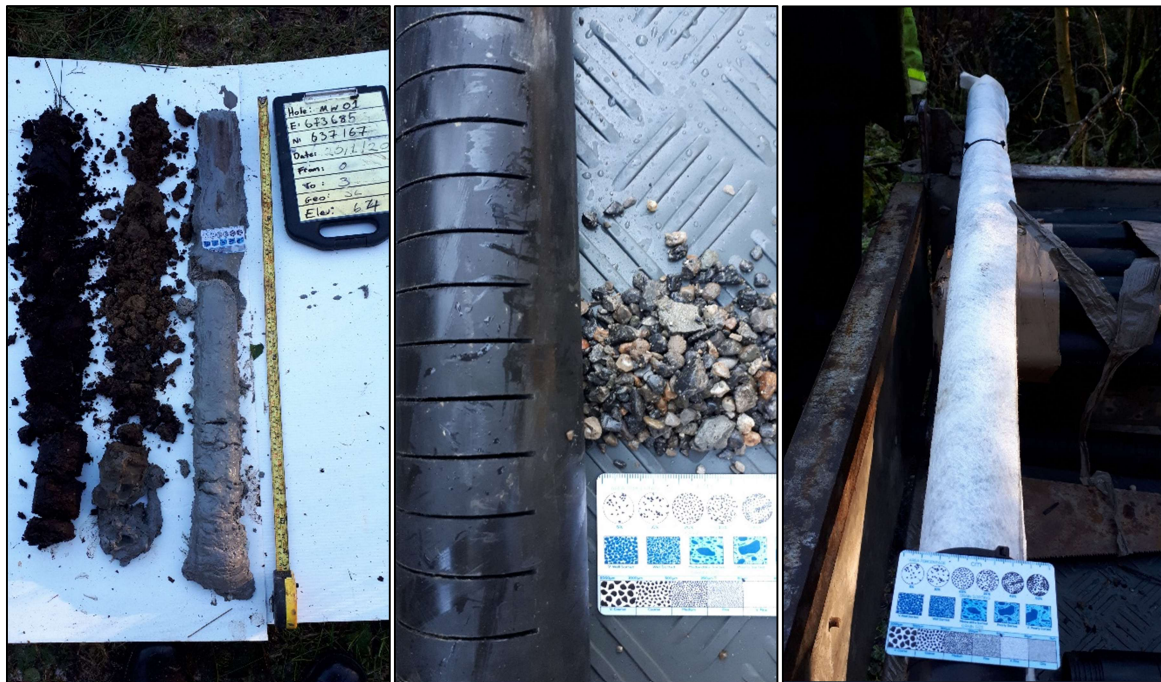
Photo 5.2-2a, 5.2-2b and 5.2-2c. Piezometer Logging and installation work.
